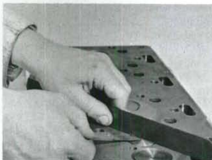
Fig. 23 — Use a straight edge and feeler gage to check valve head height. Refer to paragraph 30.
