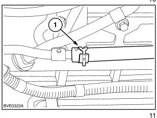
13. Disconnect the steering sensor electrical connector (if fitted).
