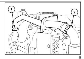
Loosen the clamp (1) and remove the air cleaner inlet.
