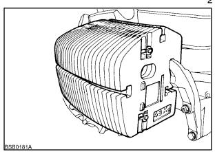
4. Loosen the hose clamps (1), remove the pipe clamp retaining bolt (2) and remove the air cooler outlet pipe.
