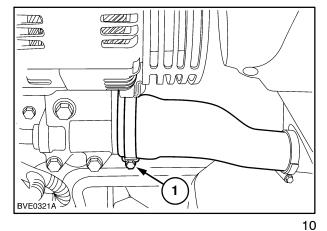
12. Loosen the coolant hose clamp (1) and disconnect the coolant hose connecting the cab heater to the radiator.
