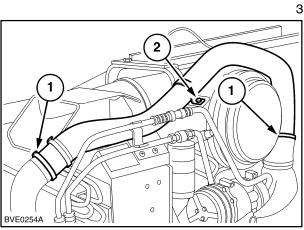
5. Loosen the pipe clamp (1), hose clamp (2) and remove the air cooler inlet pipe.
