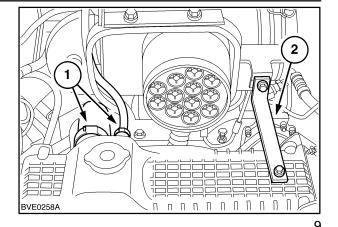
11. Loosen the hose clamp (1) and disconnect the coolant hose.
