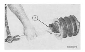
**3.** Use a brass bar and hammer to push shaft (2) through the roller.
