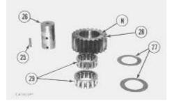
**21.** Drive spring pin (25) into planetary shaft (26) with a hammer and a punch.
