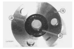
18. Using a screwdriver, remove retaining ring (22). Remove sun gear (23) from the carrier.
