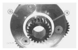
**NOTE:** Spacer (16) may remain with carrier assembly (15), or it may remain with carrier assembly (24) (see Step 19).
