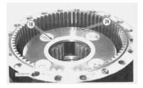
19. If spacer (16) was not removed in Step 14, remove it from carrier assembly (24) at this time.
