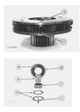
15. Drive spring pin (17) into planetary shaft (18) with a hammer and a punch.
