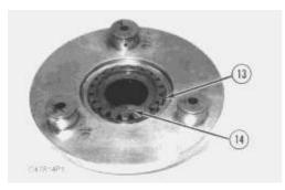
**12.** Using a screwdriver, remove retaining ring (13) from the carrier. Remove sun gear (14) from the carrier.
