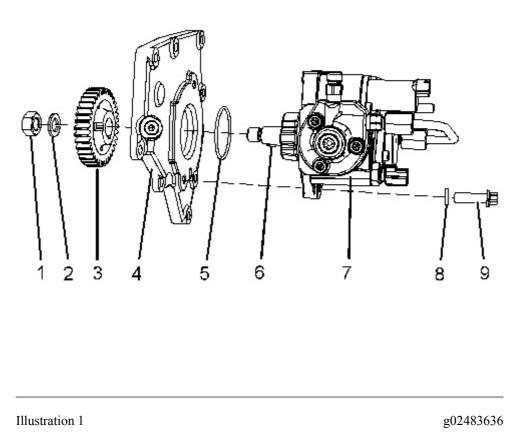
1. Use a suitable tool in order to prevent fuel injection pump gear (3) from rotating. Ensure that the gear is not damaged as nut (1) is loosened.
