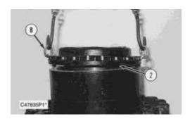
**5.** Using a soft faced hammer, break the seal between cover (2) and the ring gear. Fasten Tooling (B) and a hoist to cover (2) as shown. Remove the cover. The weight of the cover is **30 kg (66 lb)**.
