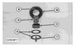
**15.** Drive spring pin (17) into planetary shaft (18) with a hammer and a punch.
