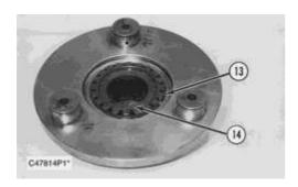
**12.** Using a screwdriver, remove retaining ring (13) from the carrier. Remove sun gear (14) from the carrier.
