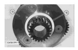
**NOTE:** Spacer (16) may remain with carrier assembly (15), or it may remain with carrier assembly (24) (Refer to the Step 19).
