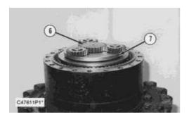
**8.** Remove sun gear (6). Remove carrier assembly (7) by lifting it straight up. The weight of the carrier assembly is **14 kg (30 lb)**.
