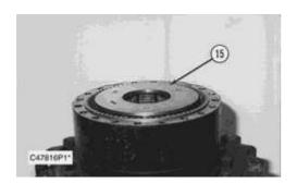
13. Using two persons, remove carrier assembly (15) by pulling it straight up. The weight of the carrier assembly is 25 kg (55 lb).
