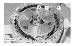
**3.** 3. Remove the bottom half of the axle housing group from Tool (G). Install axle shaft assembly (2) on Tool (G) with planetary carrier assembly (5) facing up as shown.
