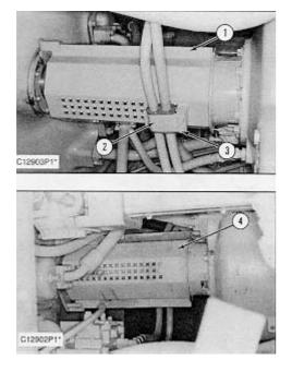
2. Remove two bolts (3) and clamps (2). Move the hoses away from guard assembly (1).
