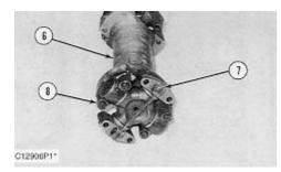
8. Remove four bolts (8) and bearing (7) from each end of drive shaft (6).
