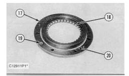
3. Install two 3/8 in - 16 NC guide bolts in the main frame case and install cage (17).
