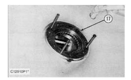
**13.** Install three 1/2 - 13 NC forcing screws in cage (17). Tighten the forcing screws evenly and remove the cage.
