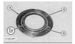
12. Remove O-ring seal (16) and seal (15) from cover (14).
