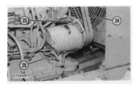
15. Loosen bolts (23) and (25), and release the tension on v-belts (24).
