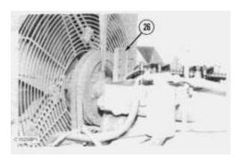
**16.** Install a nylon strap and hoist to support fan and fan drive assembly (26) as shown. Remove the four bolts that hold the fan drive to the cylinder head assembly. Rest the fan against the radiator cores and on the lower fan guards.
