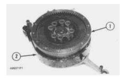
1. Remove brake band (2) and outer drum (1) from the steering clutch.
