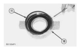
11. Remove retaining ring (11) from bearing cage (10).
