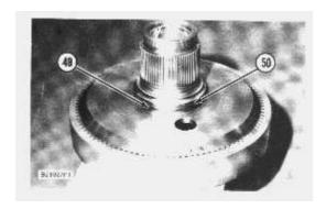
**45.** Remove seal ring (49) from carrier (50).
