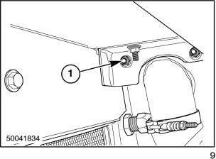
22. Disconnect wire harness at both sides of intake air heater, 1, if so equipped, and at oil pressure switch, 2.
