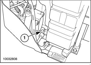
7. Loosen and remove the drain plug, 1, from the power steering reservoir, 2, and drain into a suitable container.
