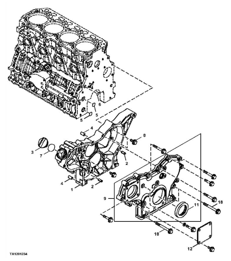
John Deere > Turf And Utility >LOADER, SKID-STEER >4TNV86CHT - LOADER, SKID-STEER >317G Compact Track Loader (PIN: 1T0317G\_\_\_J288093-) >04 ENGINE AT416882 >0443 FINISH ASSEMBLY, ENGINE >ST845458 - GEAR HOUSING
