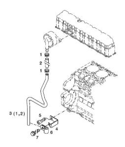
Section: B0 - ENGINE **BLEEDING TUBE**
