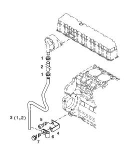
Section: B0 - ENGINE **BLEEDING TUBE**
