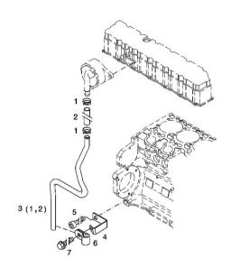
Section: B0 - ENGINE **BLEEDING TUBE**
