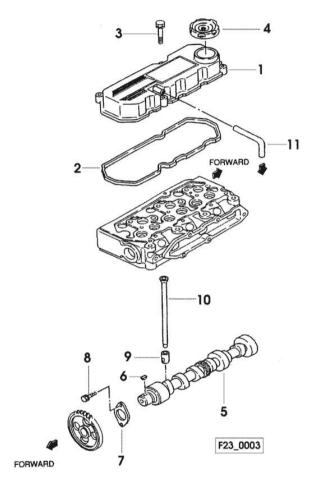
Section: ENGINE CAMSHAFT
