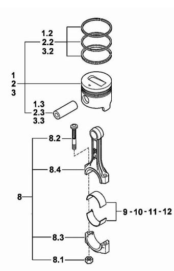
Section: B0 - ENGINE PISTON - CONNECTING ROD
