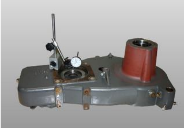
Adjusting the bearing
