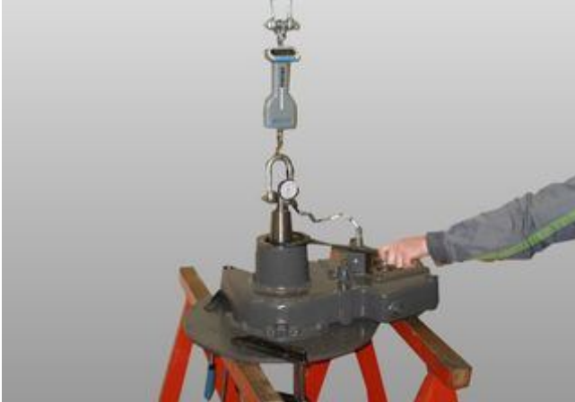
Adjusting the bearing
