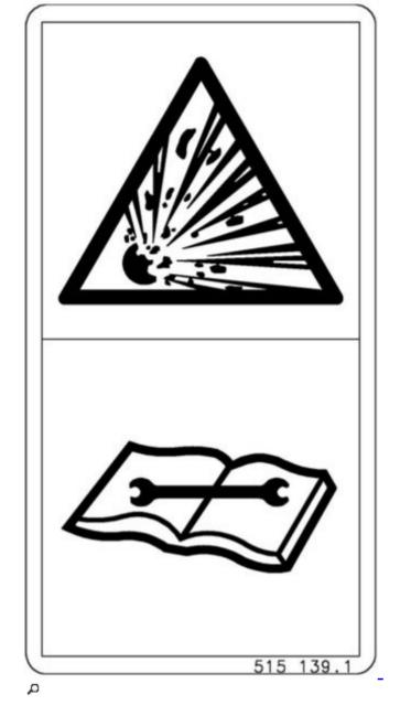
Accumulators are under gas and oil pressure. Remove and repair only according to the instructions in the Repair Manual.
