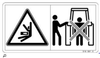
When actuating the power lift, stay outside of the lifting range of the three-point hitch.
