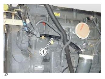
► Remove wiring loom (1) from the engine.
