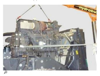
► Lift the diesel engine out of the machine.
