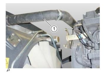
► Remove hose (1) and plug the openings tightly.
