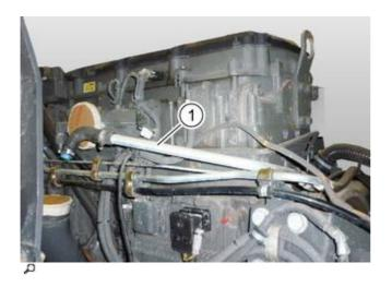
► Remove pipe (1) and plug the openings tightly.
