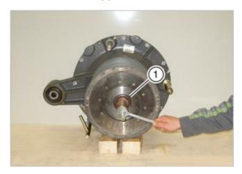
► Force in bearing (1) with an auxiliary tool.
