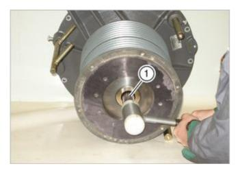
► Drive out shaft (1) with a plastic-tip hammer.
