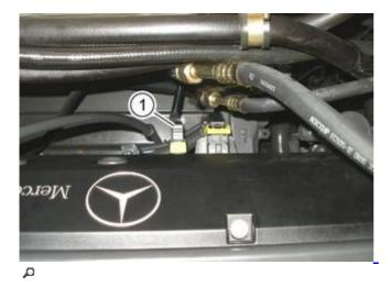
Unlock and disconnect cable connector (1).
