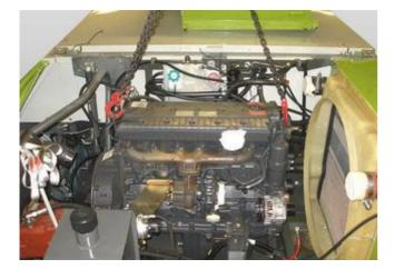
▶ Lift the diesel engine out of the machine. Caution! When lifting the diesel engine, avoid damaging any hoses and cables. Collect any escaping coolant and dispose of it.
