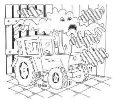
■ Do not run the engine in closed premises without adequate ventilation as exhaust fumes are deadly.
