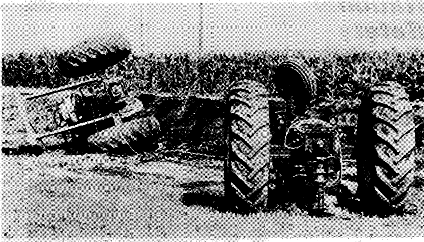
Two deliberate overturns demonstrate the safety advantage of roll-over protective systems (ROPS). The tractor without ROPS completely rolled over. The operator probably would have been killed. The frame-equipped tractor's roll was limited to 90° degrees.
