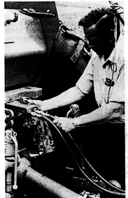
Be sure all hydraulic lines are in good condition and fit snugly. Sudden failure could cause loss of control of an implement or attachment or someone could be sprayed with hot fluid.
