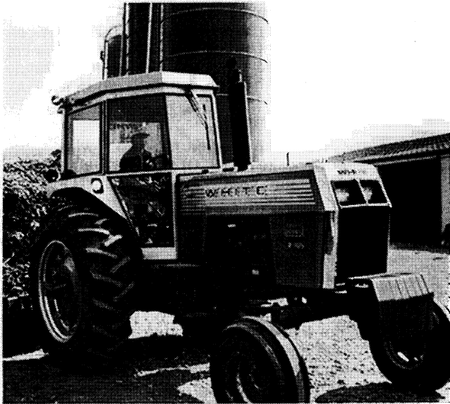
Modern tractors can do jobs more safely provided basic safe practices are followed. Operator safety is enhanced by ROPS, good lighting, front weights, and shielding danger points.
