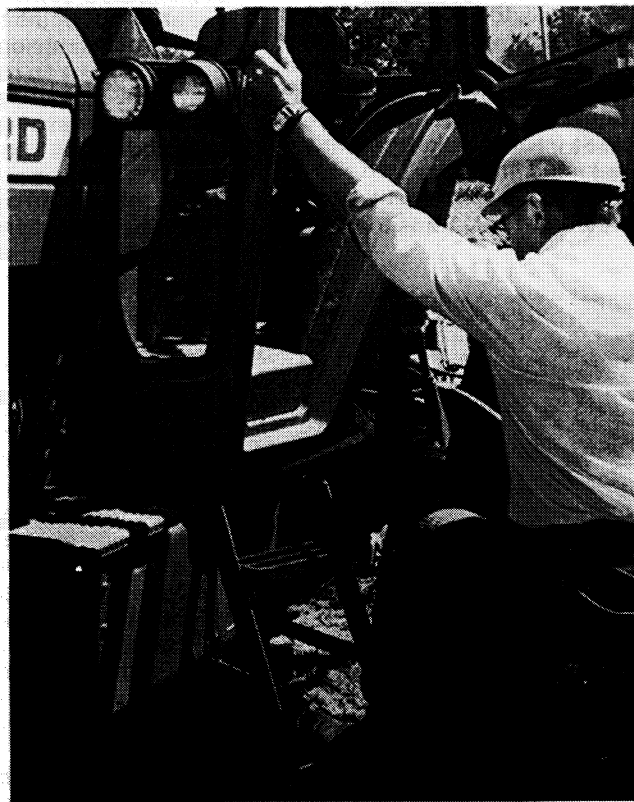
Steps and handholds make getting on and off the tractor safer and easier. Clean the steps and your shoes, before climbing aboard. Set the brakes and/or park lock before dismounting. Do not jump off.
