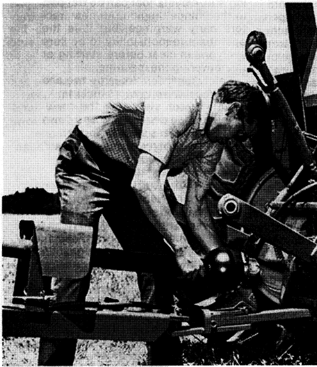
Be sure the PTO shield is free-turning before starting work and stay clear when the PTO is operating. Turn off the engine before unclogging, adjusting, or servicing PTO-driven machines. This PTO is fully enclosed for greater safety.
