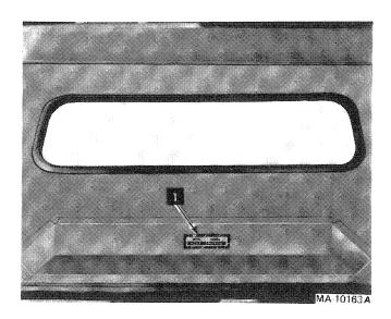
1 - Protective can serial number (behind seat) Serial Model
