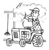
Do not operate mower in a confined area. Exhaust fumes are dangerous. Only run engine out of doors.
