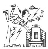
Stop engine and disconnect spark plug wire before working on mower. Stop engine before cleaning discharge chute or making any adjustments, inspection or repairs. Disconnect spark plug wire to prevent accidental starting.
