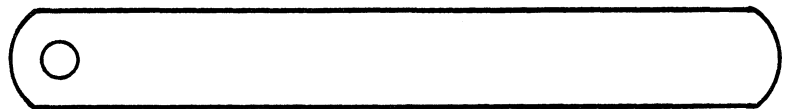
(1) Feeler Gauge (Keep for possible readjustment of electric P.T.O. clutch-See ADJUSTMENT AND SERVICING SECTION)
