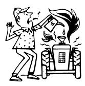
Store gasoline safely. Store gasoline in an approved tightly sealed container. Refuel outdoors and only with engine stopped. Do not spill gasoline on a hot engine.
