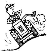
Reduce speed on all side slopes and sharp turns to prevent tipping or losing control.
