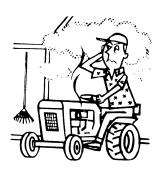
Do not operate mower in a confined area. Exhaust fumes are dangerous. Only run engine out of doors.
