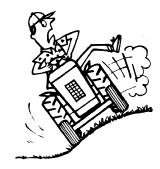
Reduce speed on all side slopes and sharp turns to prevent tipping or losing control.
