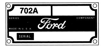
The serial no. plate is located on the front of the crossmember of the subframe. It is riveted on and should not be removed.
