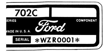
The serial number plate is located at the front of the forward frame. Record the model and serial number of your front blade.
