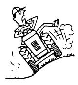
Reduce speed on all side slopes and sharp turns to prevent tipping or losing control.
