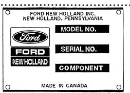
THE SERIAL NUMBER PLATE IS LOCATED ON EACH ATTACHMENT. IT IS RIVETED ON AND SHOULD NOT BE REMOVED.
