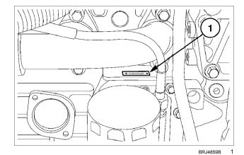
**NOTE:** The engine serial number is repeated on the information plate located on the left side of the engine oil pan.
