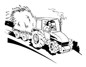
When towing, do not negotiate curves with the differential lock engaged as this may prevent you from steering the tractor.
