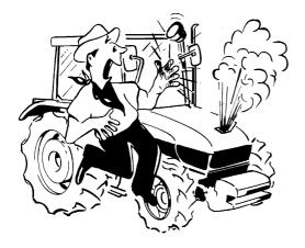
Only remove the radiator cap after the engine has been allowed to cool. With the engine switched off, use a cloth to slowly unscrew the cap and release the pressure before completely removing the cap.
