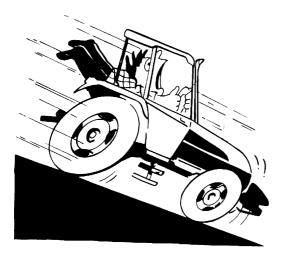
When travelling downhill, keep the tractor in gear. Never release the clutch and never leave the gears in neutral.
