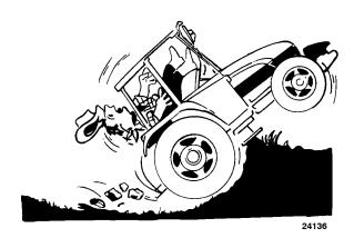
■ Engage the clutch slowly: if engaged too quickly, especially when the tractor is getting out of a hole, ditch or operating on muddy ground or steep slopes, the tractor may overturn.
