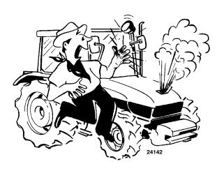
■ Only remove the radiator cap after the engine has been allowed to cool. With the engine switched off, use a cloth to slowly unscrew the cap and release the pressure before completely removing the cap.
