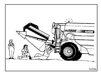
17. Do not work around the combine in loose clothing that might catch in any of the moving parts.
