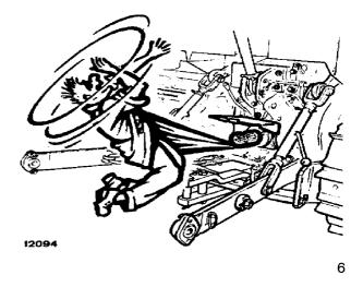
Do not wear loose clothing that may be trapped in moving parts. Check that all rotating parts connected to the power take-off are correctly protected. Thank you so much for reading. Please click the "Buy Now!" button below to download the complete manual.
