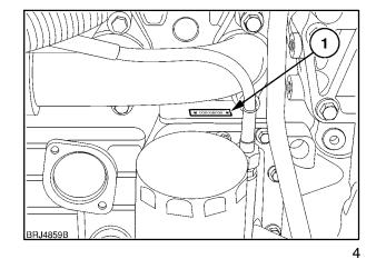
The details are repeated on the information plate located on the left side of the engine oil pan.
