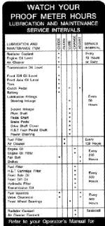
Lubrication and Maintenance Intervals PART NO: SBA390199311 LOCATION: Underside of Hood Thank you so much for reading.
