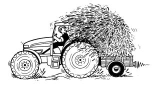
6. On four wheel drive tractors, the drive to the front axle is automatically engaged, to provide four wheel braking, when both footbrakes are applied. Owners should be aware of the effectiveness of four wheel braking which greatly enhances braking performance. Appropriate care should be exercised during hard braking.
