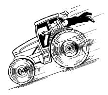
8. Keep the tractor in the same gear when going downhill as would be used when going uphill. Do not coast or freewheel down hills.
