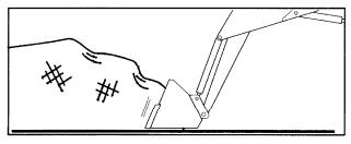
Loaders with 1-lever control, ease lever back and toward you to lift and curl bucket.
