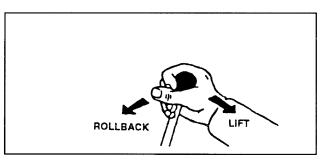
Loaders with 2-lever controls, ease both levers of tractor remote valve back to lift and curl bucket.
