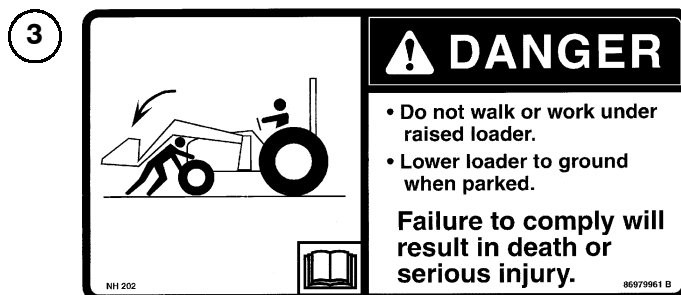
DANGER Decal Part No.: 86979961 Location: Lower loader boom
