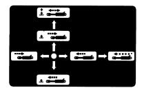
Optional) Operating Remote Control Valve-Double Spool PART NO: 86532911 LOCATION: Cover of 2-Spool Remote Valve
