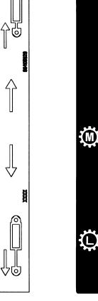
Operating Rear Remote Control Valve-Single Spool PART NO: 86405829 - Brown #3 Valve LOCATION: Right Control Quadrant
