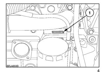
The engine serial number is repeated on the information plate located on the left side of the engine oil pan.
