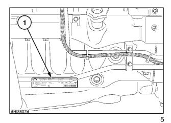
Further information relating to engine adjustments and emission level compliance are also shown on the engine information plate.
