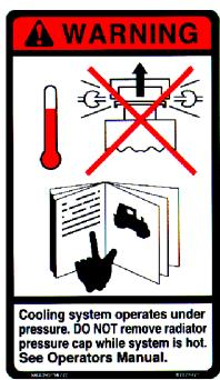
**WARNING:** Cooling System Under Pressure
