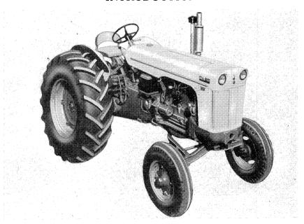
The Case 700 Series Tractor is powered by a rugged four cylinder spark ignition engine which features heavy duty precision type construction, usually found only in diesel engines. This engine is noted for its quiet operating characteristics and economy of operation.
